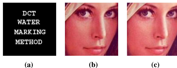
Figure 4.4: (a) Sample watermark signal (b) Host image (c) watermarked image
